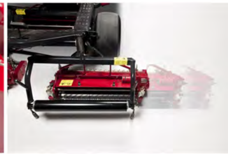
Step 3 - slide out the cutting unit
