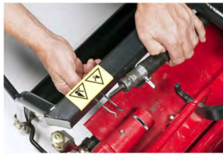
Step 1 - unclip the drive cable
