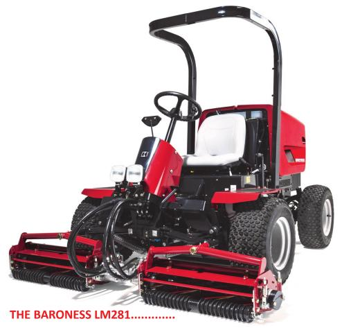
A 3-unit fine turf mower with unrivalled cutting quality The finest reel and bedknife produced in the industry Light weight combined with outstanding cutting power Low ground pressure/high traction four-wheel drive
