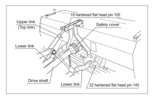
3 Attach the upper link (top link) of the tractor to the machine with "19 flat head pin 100 (1-3)," and adjust the upper link so that the machine will be almost horizontal.
