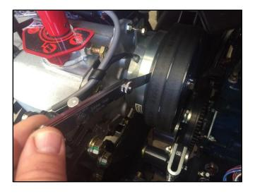
The electromagnetic clutch engages gradually in a series of pulses so as not to shock load the flexible drive cables.
