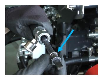
When replacing the inner drive cable only, make sure that there is just one spacer collar on the flange end as shown.
