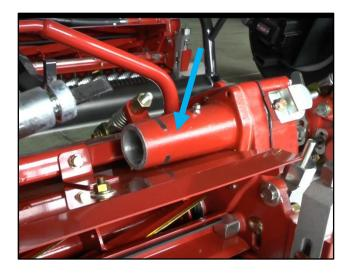
When the flexible drive cable housing socket becomes very worn and the cable fit becomes very loose then the housing socket must be replaced.
