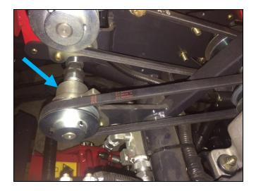
Regularly check the condition of the Belt Housing Bearings.
