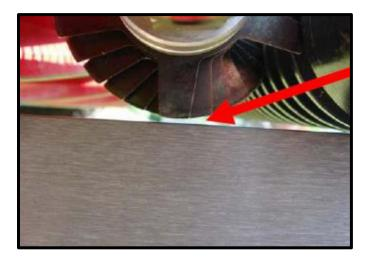
A groomer is not a ground engaging attachment and should never come into contact with the soil layer.
