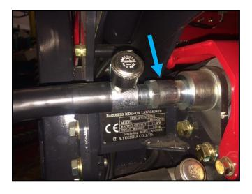
Always make sure that the outer cable retaining nut is kept tight. If it is allowed to get loose, then the flared flanged can wear through and break the inner cable.
