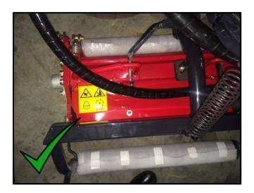
The cables should be routed with a long smooth curve and must not be able to rub or get trapped by any other component.
