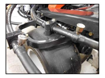
The LM315GC drive cables should have a service life of about 750 hours.
