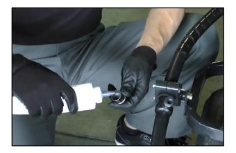
The caps of the grease reservoirs should be filled with **Bentone** thickened **Molybdenum Disulphide grease** as soon as they become empty and cannot be screwed down anymore.
