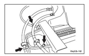
Each of the three grease reservoir caps nearest to the cutting unit end of the drive cables need to be twisted by ½ of one turn **every day** before operation. This will inject the correct daily amount of grease into the lower end of the drive cables.
