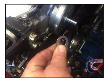
Remove 1 shim and then replace the drive pulley.
