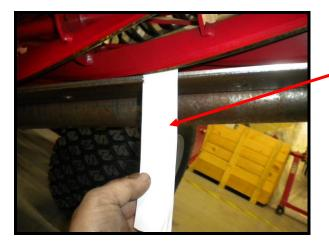
Check the cut again by using a strip of paper as previously explained. Check both ends of the blades and not just in the middle. Once again please remember to never put your hand into the cutting cylinder.
