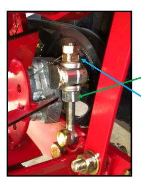
Once the top locking nut is loosened you need to lower the cylinder down slightly onto the bottom blade.
