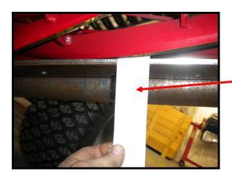
To check that the blades are cutting correctly, use a strip of paper as shown.
