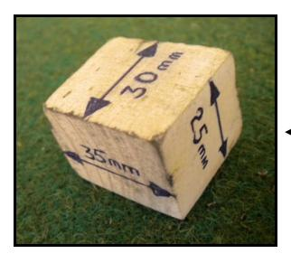
The easiest way to measure the height of cut is to make a measuring block from a piece of wood. One block can be used to measure three different heights of cut.
