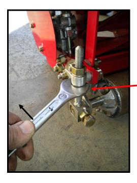
Then, in order to lower the height of cut, undo the lower adjuster nut of the rear roller assembly by rotating it clockwise. The more you undo it the more you will lower the height of cut.
