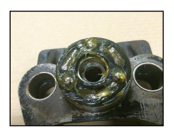
Reassemble the ball bearing activation assembly and apply new clean high temperature grease.
