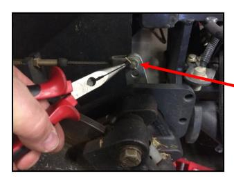
Remove the split pin, clevis pin and the associated washer that connect the brake lever to the brake cable as shown.
