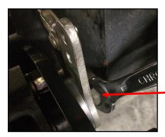
Fit the associated washers and retaining nut in the order that they were removed.
