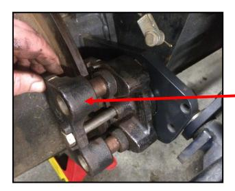
Slide the outer calliper half over the sliding pin/bushes as shown.
