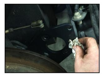
Clean the calliper mounting plate ready for re-assembly.
