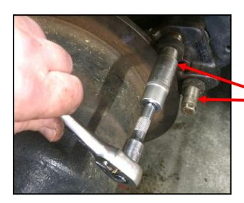
Undo and remove the two sliding bush bolts as shown.
