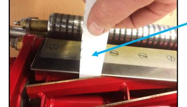
Check the cut again by using a strip of paper as previously explained. Once again please remember to never put your hand into the cutting cylinder.
