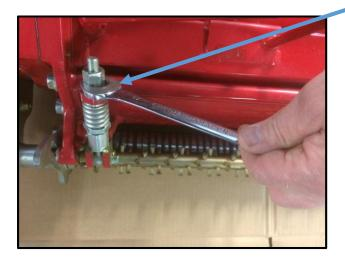
Once the blades are cutting paper on both sides you need to check that you do not have excessive blade contact.
