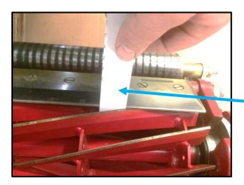
If the paper is not cut you will need to move the bottom blade towards the cutting cylinder.
