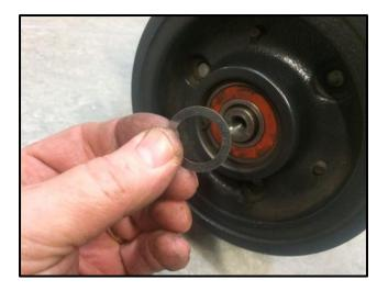
Store all removed shims on the outside of the drive pulley on the clutch shaft for future use.
