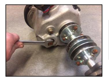
Locate the pulley shaft stub on the opposite side of the gearbox to the clutch.
