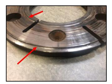
Once the drive pulley is removed you will see the clutch pressure plate.
