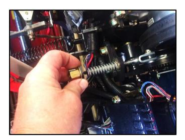
Remove the spring tensioning nut from the threaded tension adjuster rod.
