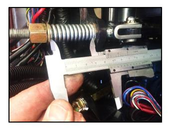
Tighten the adjusting nut until the tension spring reaches a length of 45mm.
