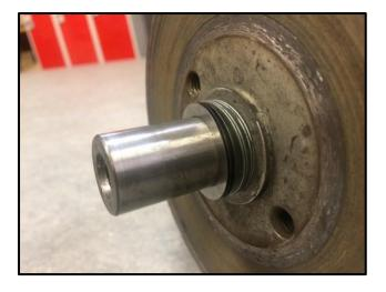
Before adjusting the clutch, clean the clutch shaft using some fine abrasive paper.
