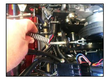
Remove the tensioning spring and its associated washers from the threaded adjuster rod.
