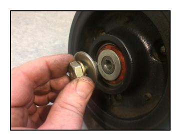
Refit the pulley retaining screw and washers to the clutch shaft as shown.
