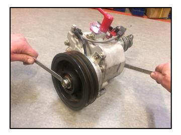
Holding the back end of the clutch shaft with a 17mm spanner, tighten the pulley bolt using another 17mm spanner.
