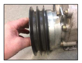
Rotate the pulley by hand.
