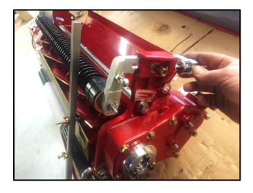
Adjust the height of cut to the customers desired setting.
