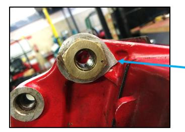
Insert the bronze cam bushes so that the marker dot on the bush aligns with the pointer on the mower frame as shown.
