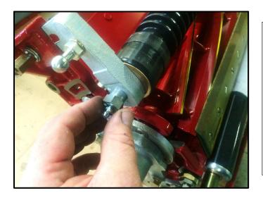
Screw in the shouldered roller bolt as shown and tighten with a 17mm spanner.
