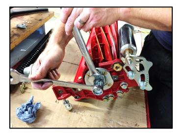
Hold the gear into position to stop it rotating using a 27mm open ended spanner on the flats found on the inside end of the gear.
