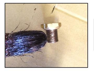
Apply a thin layer of 'Copper-Slip' to the outside surface of the bronze cam bush as shown.
