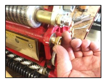
Insert the un-lubricated bronze bush into the cutting unit frame to see that it rotates freely.
