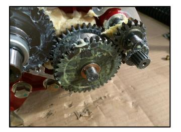
Refit the thrust washers over the gear shafts in the same order that they were removed.
