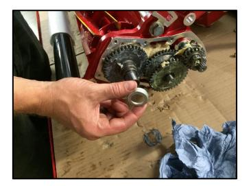
Refit the pin retaining cap over the cutting reel shaft.
