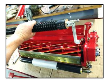
Remove the entire roller assembly as shown.
