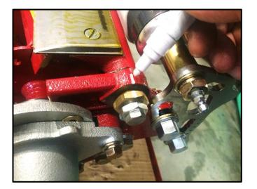
Keep adjusting the bronze cams slightly until the paper is cut cleanly on both sides of the bedknife.
