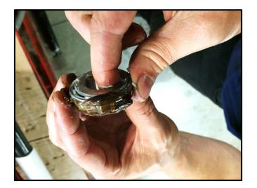
Inspect the condition of the reel bearing and replace if necessary.
