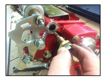
Insert the lubricated pivot pins inside of the lubricated bronze cam bushes.
