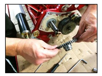
Remove the drive gear from the end of the reel shaft.
