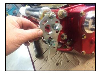
Re-set the rear roller to its desired level of aggression using the provided guidance chart.
