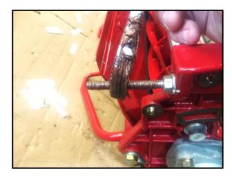
Clean the front roller adjuster threaded rods with a wire brush and then apply a thin coating of 'Copper-Slip' to them.
