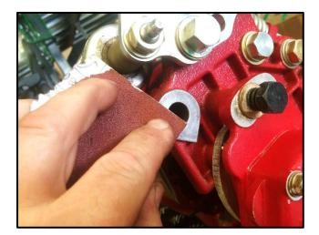
Thoroughly clean the inside and outside surfaces of both ends of the cutting frame where the bedknife carrier locates with abrasive paper as shown.
