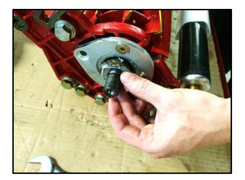
Check the condition of the reel bearing and replace if necessary.
