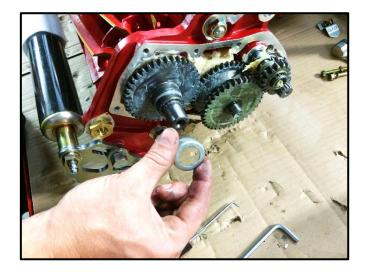
Remove the gear pin retaining cap from the cutting reel shaft.
