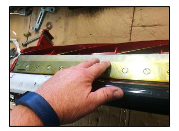
We now need to ensure that the bedknife is running parallel to the cutting reel.
