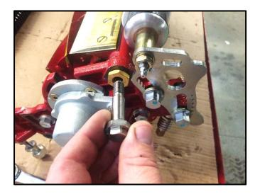
Insert the non-lubricated pivot pins through the bronze cam bush at both ends of the cutting unit.
