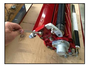
Remove the roller bracket locking nut, bolt and washers from the same side using a 13mm spanner.
