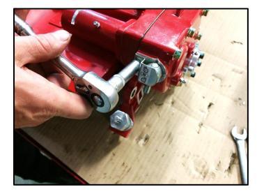
Remove the bolt that holds the reel direction selector retaining spring into position as shown.
