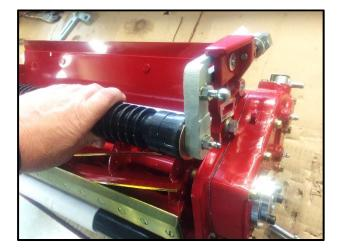
Fit the front roller onto the cutting unit on one side and secure with the coachbolt, washers and nut.
