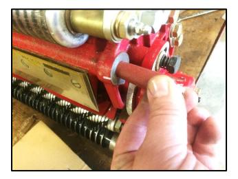
Thoroughly clean the frame inside the hole where the bronze cam bushes locate using some abrasive paper as shown.
