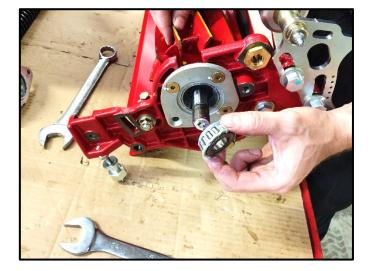
Remove the 'wave' spring washer and the cutting reel bearing from the reel shaft as shown.
