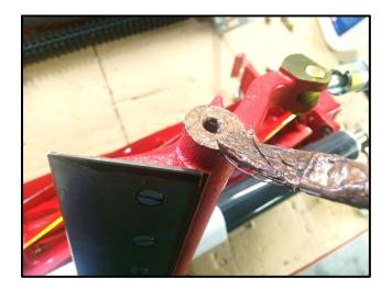
Clean up both ends of the bedknife carrier at the pivot point with abrasive paper to leave the surface clean.
