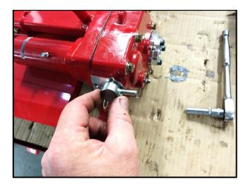
Refit the drive selector into the gearbox.
