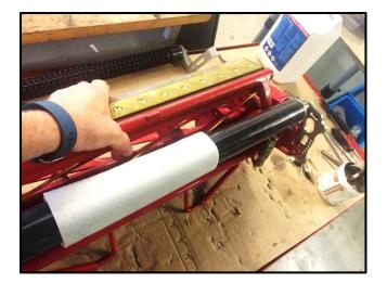
Fit the bedknife carrier assembly into position as shown.
