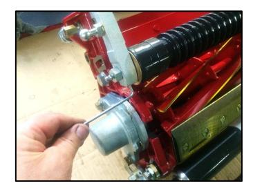
Tighten the grub-screw in the roller bracket against the shouldered bolt to lock the roller position.
