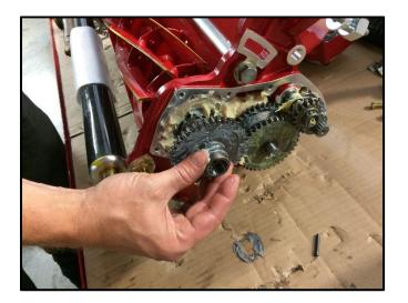
Refit the gear over the cutting reel shaft so that it locates over the drive key.
