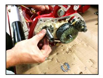
Insert the bearing over the reel shaft and into its housing.
