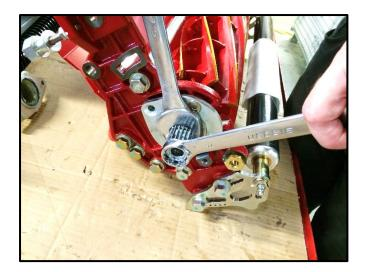
Screw the gear locking nut on to the end of the reel shaft until it touches the gear.
