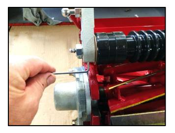
Locate the roller bracket with the shouldered roller bolt going through it.
