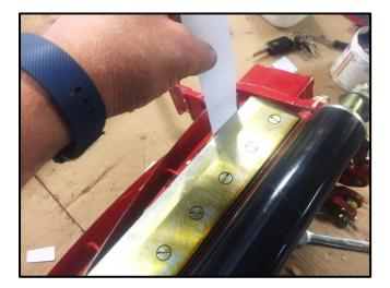
Using a piece of paper held square to the bedknife, rotate the cutting cylinder slowly whilst checking to see if the paper is being cut.
