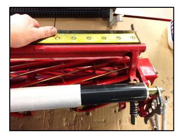
Remove the bedknife assembly from the cutting unit as shown.
