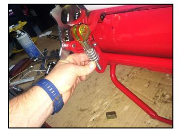
Gently move the bedknife carrier a little until you are able to get the adjuster rods to locate inside their correct frame locating hole.
