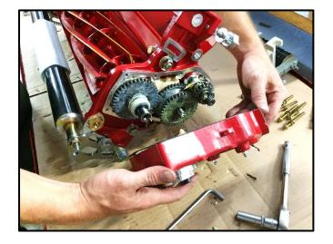
Remove the gearbox cover as shown being careful not to damage the gasket and to make a note of the location of the gear shaft thrust washers.
