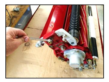
Tighten both roller bracket securing nuts as shown.
