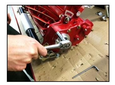
Remove all gearbox retaining bolts using a 10mm socket/spanner as shown.
