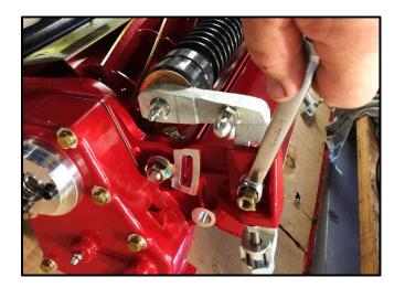
Remove the roller bracket locking nut, bolt and washers from the opposite end of the roller.
