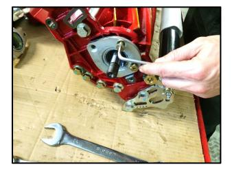
Check the condition of the oil seal located in the aluminium bearing housing and replace if necessary.
