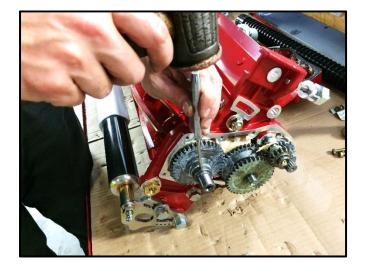
Using a small punch and hammer, remove the drive gear securing pin as shown.
