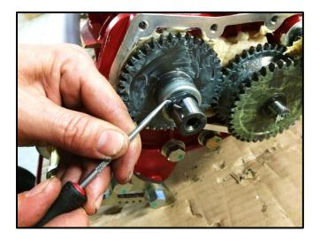
Very carefully using a pointed but blunt tool, remove the cover retaining 'O' ring from the reel shaft as shown.
