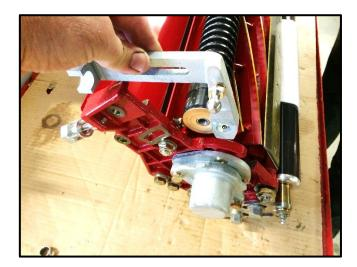
Remove the roller bracket and the brass thrust washer from the dismantled side as shown.
