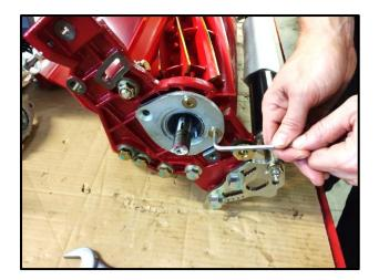
At the other end of the cutting unit, undo the 3 x M8 countersunk screws using a 5mm hexagon key.
