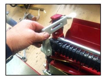
Fit the roller bracket to the other end of the cutting unit and hold it in place loosely with its securing coachbolt, washers and nut.
