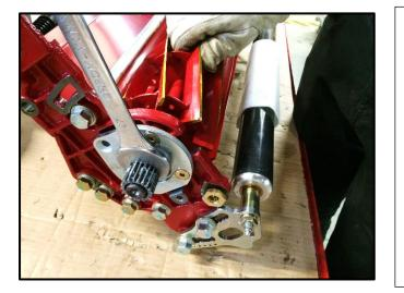
Using a 27mm spanner, tighten the attachment drive gear fully up to locate the bearings.
