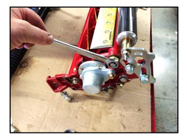
Locate the pivot pins that secure the bedknife carrier into position.
