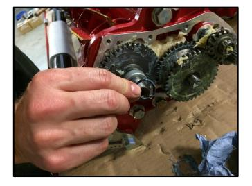
Refit the cap retaining 'O' ring over the cutting reel shaft, making sure that it is seated within its intended groove.
