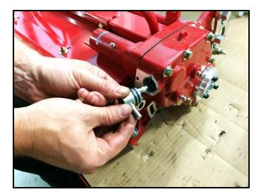
Remove the reel direction selector lever with a firm pull.
