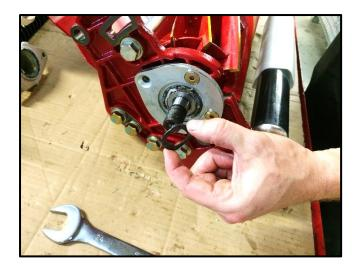
Fit the 'wave' spring washer over the cutting reel shaft so that it rests against the bearing.
