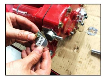
Fit the selector lever retaining spring and secure using the M6 screw.
