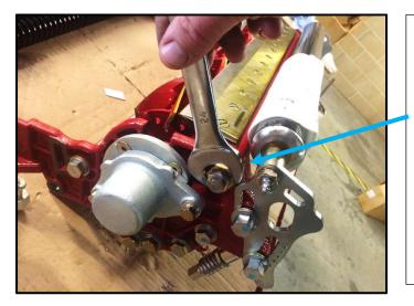
If the paper is cut at one end of the bedknife but not at the other, then we need to rotate the bronze cam bushes to achieve an even cut.
