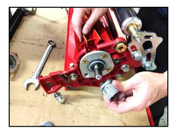
Remove the locking nut and the gear from the reel shaft as shown.
