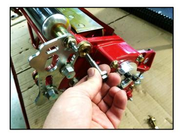
Loosen the pivot pins on both sides of the bedknife carrier using a 13mm spanner.
