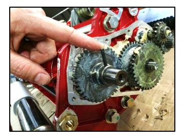
Insert the locating pin through the hole in the drive gear, gently tapping home if necessary.
