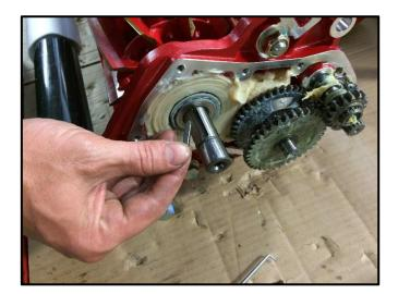
Remove the key from the reel shaft.
