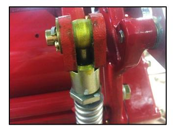
Make sure that the lugs of the spring tension collar are located within the slot of the frame as shown.
