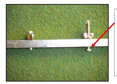
The required height of cut needs to be set between the underside of the setting screw head and the setting bar.
