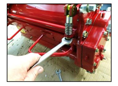
Slacken off and remove the bedknife adjuster nuts from both sides of the cutting unit as shown.
