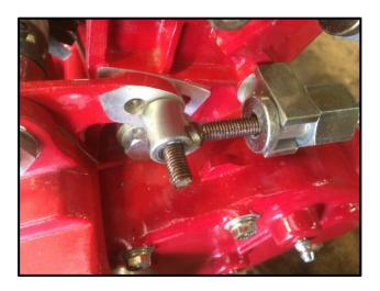
Clean the threads of the adjuster locking bolt using a wire brush.
