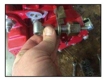
Undo the attachment adjuster position locking nut.
