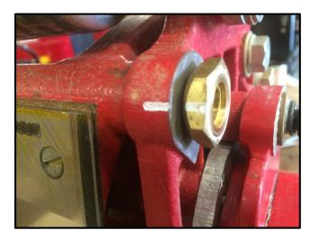
Refit the brass cam making sure that you align the original marks that were applied previously.
