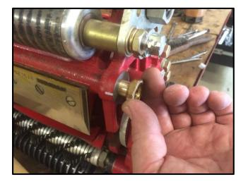
Dry fit the brass cam into the cutting unit side frame.
