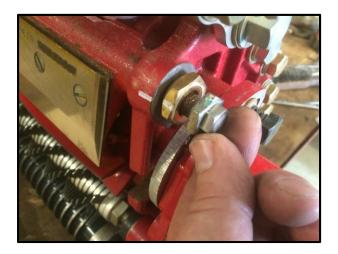
Apply a thin layer of anti-seize grease to the pivot pin to include its threaded area.
