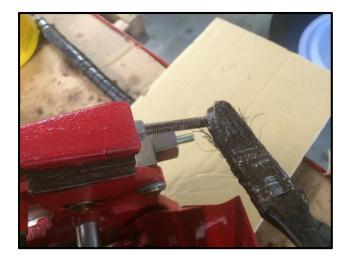
Clean the threads of the front roller adjuster rod using a wire brush.
