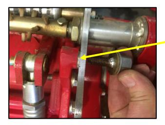
Only ever remove the rear roller bracket retaining bolts one at a time.
