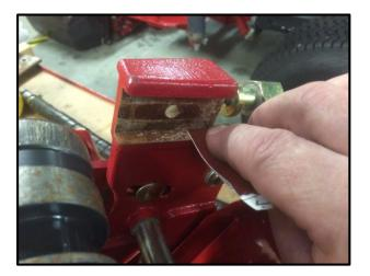
Remove the front roller assembly.
