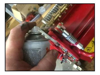
Apply some spray lubricant to the bedknife adjuster pivot pin and threaded adjuster rod/nut assembly.
