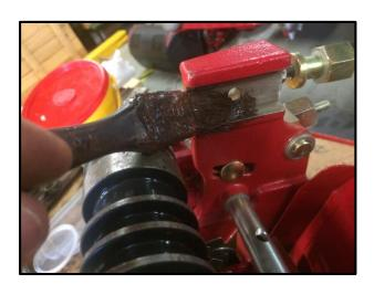
Apply a thin layer of anti-seize grease (copper-slip) to the cleaned up front roller bracket channels on the cutting unit side plates as shown.
