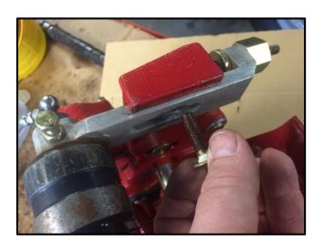
Re-assembly all cleaned and lubricated parts and adjust the height of cut as required.
