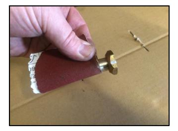
Remove the brass cam nut from the mower side case.
