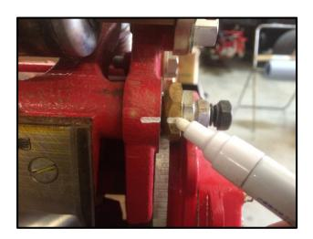
Always mark the position of the pivot pin cam against the cutting unit frame before carrying out any maintenance to this area.
