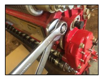
Hold the brass cam into position with a 24mm spanner so that the setting marks line up.
