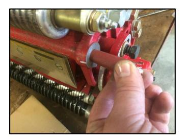
Clean the inside bore of the cutting unit side frame where the brass cam fits using an abrasive paper.
