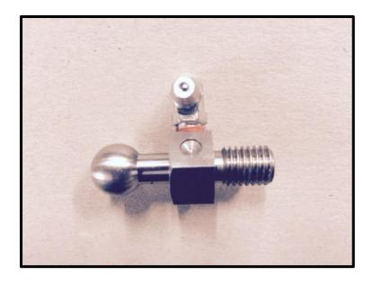
Screw the C Type grease nipple into the left mower mounting bolt as shown.
