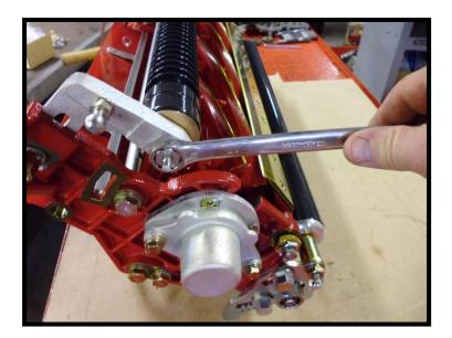
Remove the 17mm retaining shoulder bolt.
