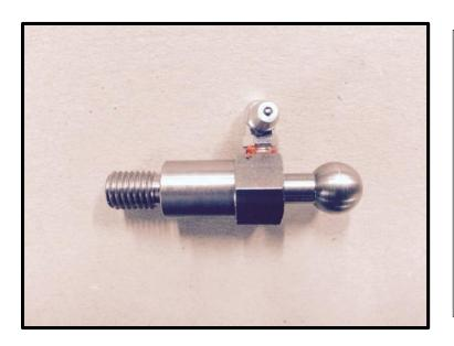
Screw the C Type grease nipple into the right mower mounting bolt as shown.
