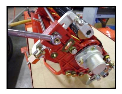
Remove the front roller assembly. Then remove the grease point adapter nut.
