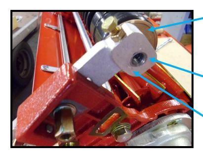
With the large thrust washer in place, fit the new straight roller bracket over the long shaft end of the roller shaft as shown. Make sure that the end of the shaft is level with or protruding outside of the aluminium bracket. If it is not then the outside face of the bracket will need to machined until it is level with the end of the shaft.
