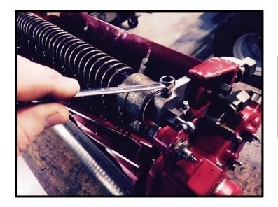
Lightly tighten the M6 locking screw to secure the position of the mower attachment bolt.
