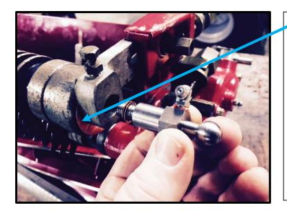
Fit the roller bracket to the other side making sure that a large thrust washer goes between the roller and the bracket. Fit the shouldered roller retaining bolt as shown using shims to make sure that the grease nipple hole is facing forwards when this bolt is tightened.
