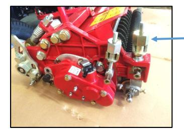
Use the height of cut adjusting nut to change the front roller to the desired setting.
