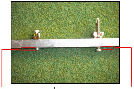
This end of this screw (as shown) needs to be adjusted so that it measures the same distance as the desired groomer setting. This screw needs to be adjusted so that the distance between the setting bar and the underside of the head of the screw (as shown) is adjusted so that it measures the same distance as the desired height of cut.
