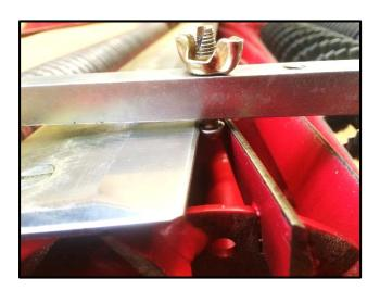
Locate the underside of the setting screw head so that it slides over or up against the top cutting surface of the bedknife.
