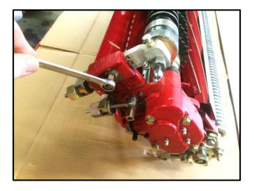
Once the desired settings is achieved, tighten the front roller bracket locking nuts using a 13mm spanner.
