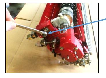
Loosen the height of cut locking nut using a 13mm spanner.
