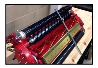
Adjust the height of cut and the groomer height as desired.
