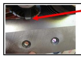
De-Thatching Blades are thicker and stronger than groomer blades and are designed to run within the thatch layer.
