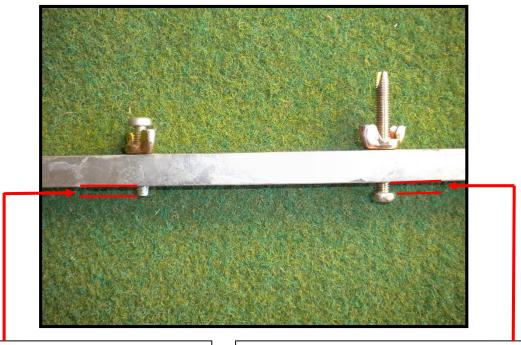
This end of this screw (as shown) needs to be adjusted so that it measures the same distance as the desired groomer setting.
