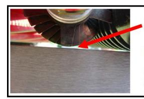
The groomer blades should never come into contact with the soil and are only designed to run between the grass leaf.
