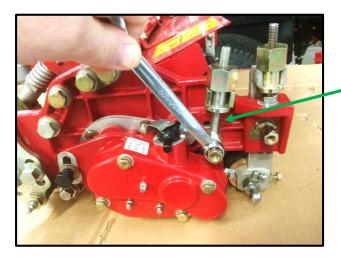
To adjuster the groomer height you will firstly need to slacken the adjustment locking nuts as shown using a 13mm spanner.
