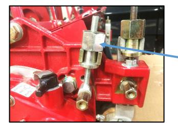
Now adjust the height of the attachment by rotating the Adjuster nut.
