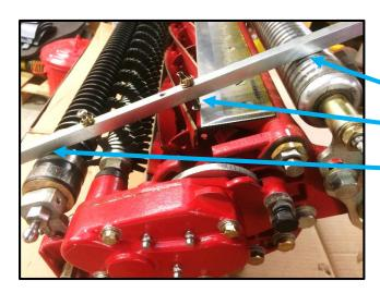
With the height of cut already set, fit the setting bar to the machine as shown so that the underside of the head of the height of cut adjusting screw is sitting on the upper cutting surface of the bottom blade and that ends of the setting bar are resting up against the rear and front rollers.
