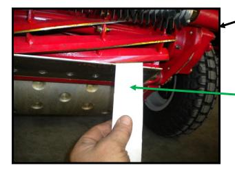
To check that the blades are cutting correctly use a strip of paper as shown.
