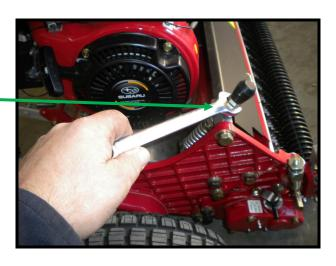
Check the cut again by using a strip of paper as previously explained. Once again please remember to never put your hand into the cutting cylinder.
