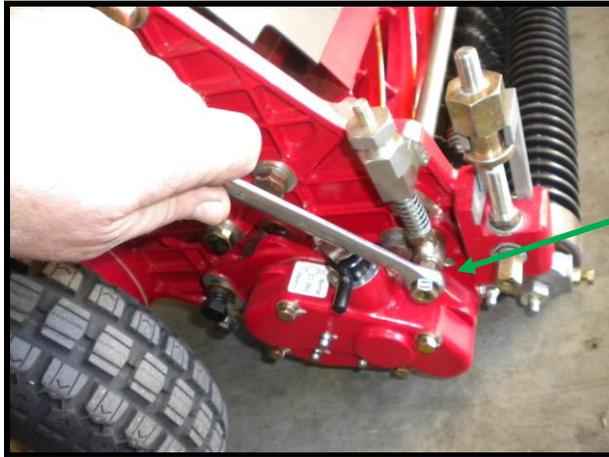
Tighten the groomer height locking nuts on both sides of the machine.
