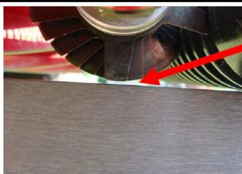
Typical Groomer height set is between **0.040" to 0.060" ABOVE** the **Roller Height** depending on the green and soil conditions.
