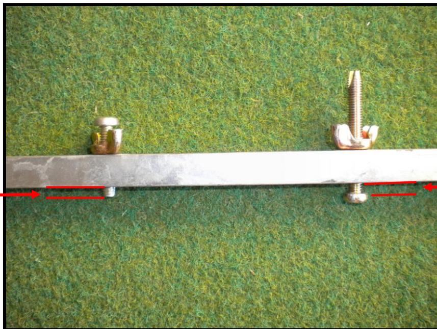
This end of this screw (as shown) needs to be adjusted so that it measures the same distance as the desired groomer setting.
