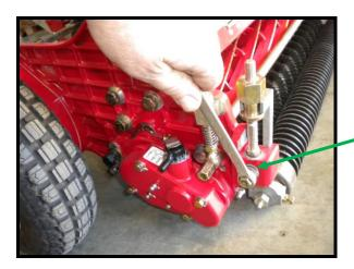
Finally tighten the roller adjuster locking nuts. After tightening these, re-check the height of cut to see that nothing has moved. If it has, then re-adjust as necessary.
