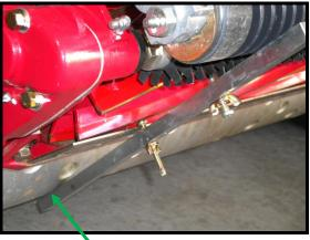
The end closest to the height adjusting screw should be resting on the rear roller as shown.
