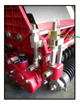
You now need to adjust the height of the front roller until the correct setting is achieved. To adjust the front roller height, twist this adjusting nut. Twisting it clockwise will lower the roller and twisting it anti-clockwise will raise the roller.
