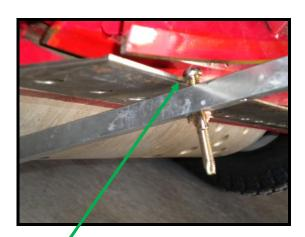
With the machine tipped back, fit the setting bar as shown with the underside of the adjusting screw head resting on the cutting edge of the bottom blade.
