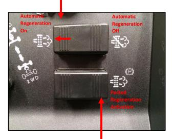
This switch is used to activate a 'Parked Regeneration' if 'Automatic Regeneration' has either been turned off due to a potential fire risk, or if the automatic system has not been able to cope with keeping the DPF clean on its own.
