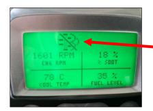
If 'Automatic Regeneration' is switched off, then this Icon is displayed on the LCD Screen.
