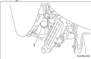
Replacement of Engine Oil Filter\_001
