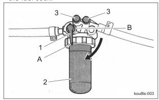
Replacement of Fuel Filter Element\_003
