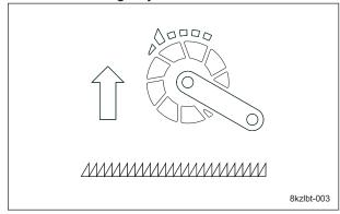
Mower Unit Up-Switch (with Reel Excess Discharge System)
