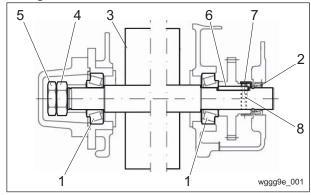
Attaching Reel Cutter (Cutting Cylinder)\_001
