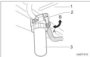
Replacement of Fuel Filter Element\_001
