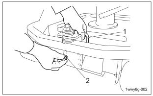
Adjustment With Cutting Height Adjusting Plates 002
