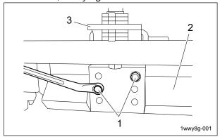
Adjustment With Cutting Height Adjusting Plates\_003
