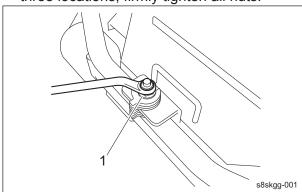
Adjustment With Adjusting Collars\_004
