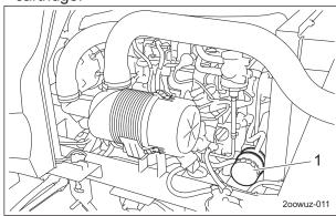
Replacement of Engine Oil Filter\_001
