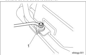
Adjustment With Adjusting Collars\_001
