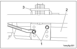
Adjustment With Cutting Height Adjusting Plates\_001
