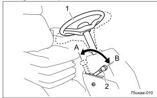
Adjustment of Steering Wheel Position\_001
