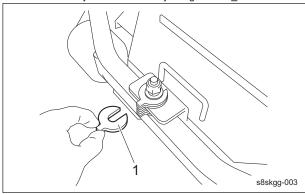
Adjustment With Adjusting Collars\_003
