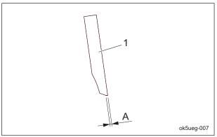
Sharpening of Reel Cutter (Cutting Cylinder) 002
