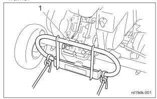
Towing The Machine in An Emergency\_001
