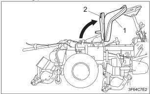
Opening and Closing of Seat Mounting Plate\_001
