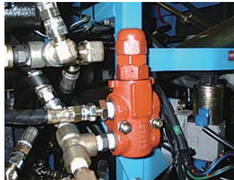
④ Relief valve Protection of gear pump
