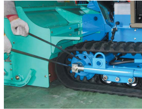
C. Detaching the rubber crawler
