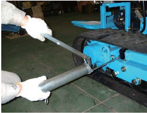
A. Stretching the rubber crawler
