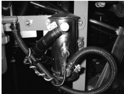
B. Fuel pump Fuel supply electromagnetic pump + Secondary fuel filter
