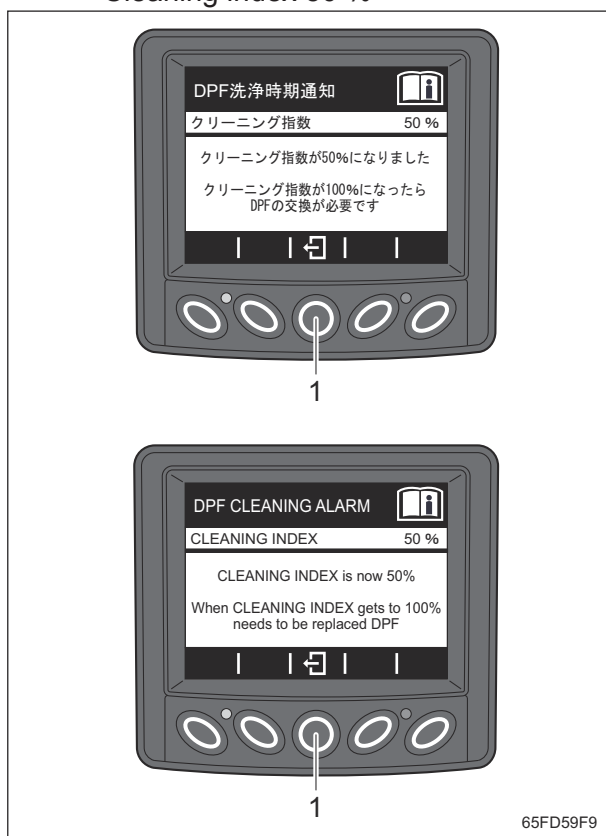
DPF Cleaning Alarm_002
